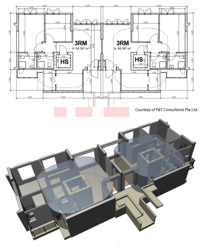
Examples of a Floor Plan and 3D view showing shelters:
