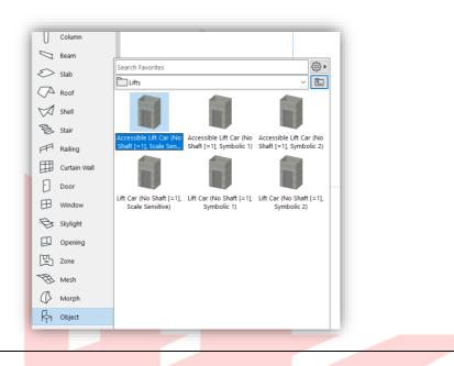
Note: The stored Favorites include the lift shaft set at a minimum thickness of 1mm. This is only necessary to make the lifts visible in their full heights when highlighted for accessibility. Actual shafts are to be built using the Wall tool and an additional Empty opening (Door tool) placed.
